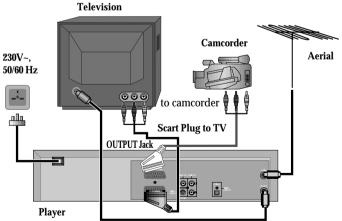
If you have connected your camcorder in this way, you can also connect a scart lead from "AV1" on the back panel of the player to the television. To use this function, see page 17.
